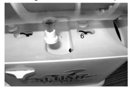
4. Pull the 2 white end plugs (front and back) out to release the aluminum/auger mixing mechanism from mixing
